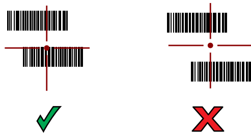
Figure 25 RS6000 Pick List Mode with Multiple Barcodes in Aiming Pattern
