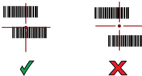
Figure 22 RS5100 Pick List Mode with Multiple Barcodes in Aiming Pattern
