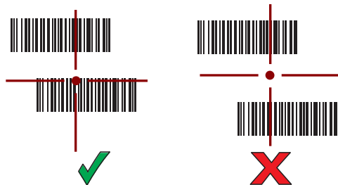
Figure 28 RS507/RS507X Pick List Mode with Multiple Barcodes in Aiming Pattern
